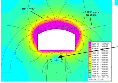
Spacers or mechanical adjustment is used to raise or lower the magnet array at specific locations <u>Magnet Array Optimization for Rotating Cylindrical Magnetrons</u> Uniformity Adjustment – Addressing "Local" Effects:
