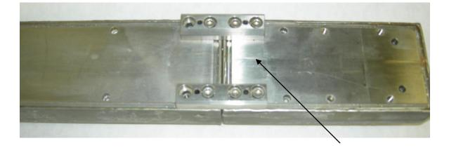
Addition of Spacers to Adjust Magnet Array to Target Surface Distance
