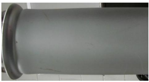
End Grooving refers to the target erosion at the racetrack turnarounds
