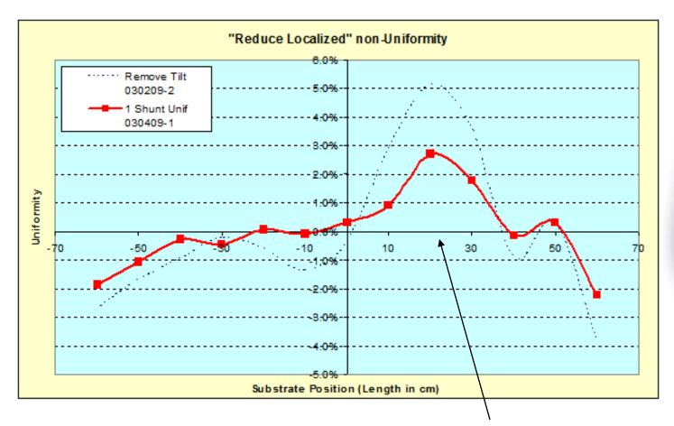
The addition of a single shunt brought the total uniformity in the correct direction but was not strong enough. Add 2<sup>nd</sup> shunt to other side of magnet array!
